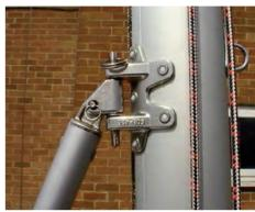
2:3 Having fixed the boom and gnav to the mast you can thread the gnav control line.
