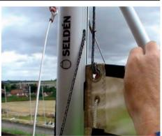
5:4 Cleat the main halyard in the cleat on the left of the mast. Sweat the halyard in order to make sure that the sail is at the top of the mast.
