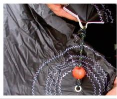
4:15 Pull on the end of the spinnaker halyard coming from the end of the spinnaker chute within the boat in order to pack the spinnaker into the chute.
