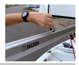
5:6 Pass the outhaul through the eyelet in the clew, and then back to the end of the boom, where the end of the outhaul should be cleated.
