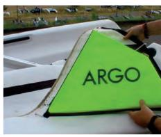
5:2 Tie the free end of the main halyard to the eyelet on the top of the mainsail.
