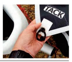
4:12 Temporarily remove the red ball from the spinnaker halyard. Then pass the end of the spinnaker halyard through the eyelet in the sail as shown.
