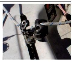
The tail of the jib halyard can be stowed in the pocket on top of the spinnaker chute. It is not advisable to leave the jib up overnight, and always take the jib tension off when the boat is not being sailed.
