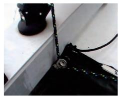
4:3 Take the free end of the halyard through this cleat; it is underneath the spinnaker chute, and it may need to be moved for the pulley to be exposed.
