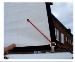
6:3 From the top eyelet, the reefing line comes back down to the boom. Tie a stopper knot in the end of the line, and then slide the knot into the cut out in the boom.
