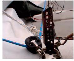
1:5 Fix the base of the mast to the mast step on the cross beam with the pin and ring from the mast step.
