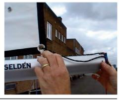
5:7 Hook the downhaul onto the sail, ensuring that it is not twisted before applying any tension.
