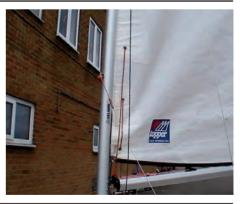
6:5 Release the main halyard from the cleat, and uncleat the gnav, and then pull on the reefing line.
