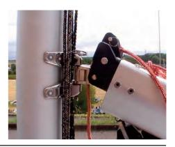
2:2 Next attach the strut to the upper fitting on the mast. Ensure the toggle is correctly orientated as per the Selden/Superspar info sheet.
