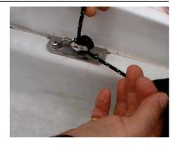
4:6 Pass the halyard through this eyelet in the bottom of the spinnaker chute.
