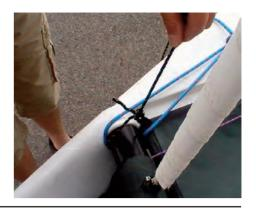
4:2 Take the other free end of the halyard and take it through this pulley on the front of the cross beam.
