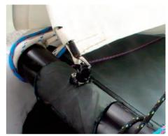
TIP: Wrap some electrical tape around the furler. This will protect the spinnaker from the sharp split ring and help to prevent rips in the sail.
