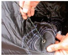
4:13 Then re-attach red ball to spinnaker halyard on the other side of the sail.
