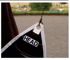
4:10 Tie the spinnaker sheets onto the CLEW of the spinnaker.
