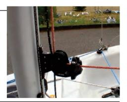
2:4 Now thread the mainsheet. Starting from the centre cleat on the hull (NB: ensure the the ratchet clicks when the rope is pulled in), go up to the rear block, and thread the line back to front. Then go to the pulley on the two thin lines, and thread it back to front.
