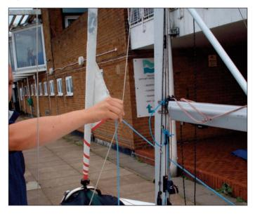
The tail of the jib halyard can be stowed in the pocket on top of the gennaker chute. It is not advisable to leave the jib up overnight, and always take the jib tension off when the boat is not being sailed.
