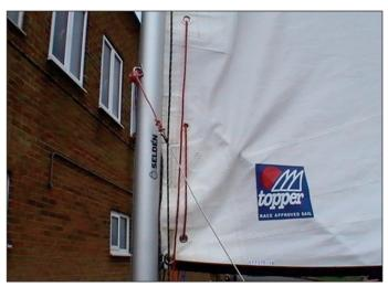
6:5 Release the main halyard from the cleat, and uncleat the gnav, and then pull on the reefing line. The foot of the sail should fold up so that the sail area is reduced. Once the desired sail area is achieved, cleat the reefing line and main halyard, and re-apply gnav tension.
