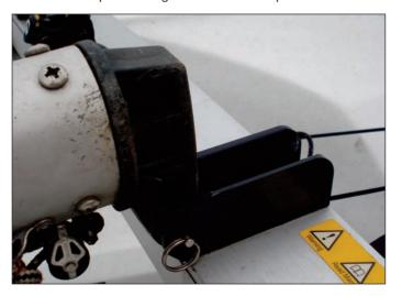
1:6 Pull the mast up using the forestay. To make it easier, someone else can lift the top of the mast.
