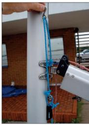
2:4 Now thread the mainsheet. Starting from the centre cleat on the hull (NB: ensure the ratchet clicks when the rope is pulled in), go up to the rear block, and thread the line from back to front. Then go to the pulley on the top of the centre block, and thread it from back to front. Then go to the front pulley on the boom, and thread it from front to back.
