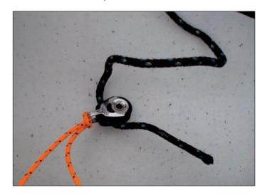
4:6 Pass the halyard through the eyelet in the bottom of the gennaker chute.
