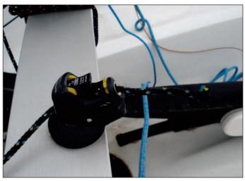
4:5 Take the halyard back through the pulley on the line (attached under the thwart) next to the back of the centreboard.
