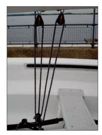
2:5 The mainsheet goes to the pulley on the deck and through the hole in the centre of the pulley. Tie a stopper knot to prevent the line unthreading. Tie a figure of eight knot in the loose end so that the boom does not hit the shroud when sheeting out.
