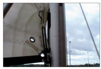
6:1 Pull on the red reefing line so that it comes out of the boom some way.
