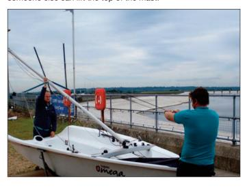
1:7 Having pulled the mast upright, secure the forestay around the stainless steel chute mouth bar. Ensure all halyards are clear and not twisted.
