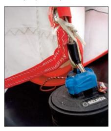
3:2 Do the same for the head of the jib onto the furler on the jib halyard. Again, wrap some tape around it.
