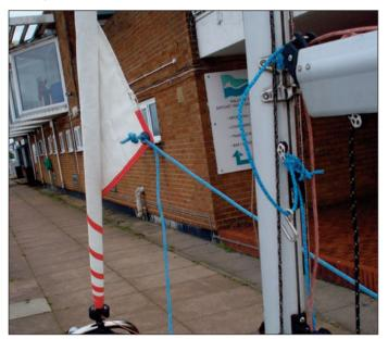
3:8 Cleat the jib furler off in the cleat underneath the crossbeam.
