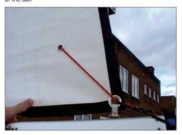
6:3 From the top eyelet, the reefing line comes back down to the boom. Tie a stopper knot in the end of the line, and then slide the knot into the cut out in the boom.
