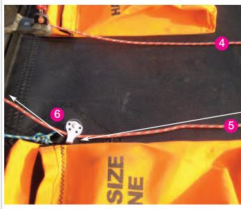
G. (7) Then feed spinnaker halyard into back of spinnaker sock.
