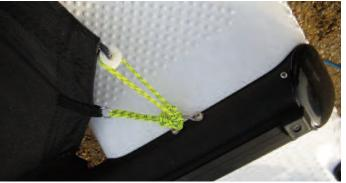
Then repeat on opposite side. Ensure trampoline is as taut as possible to ensure a firm platform.
