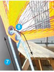
F. Untie tail end of jib halyard and tie one end off loosely onto the bridle eye (F).
