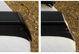
B. Remove slugs from front beam.
