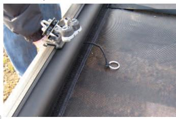
E. Feed spinnaker halyard (4) back along trampoline, through steel ring.
