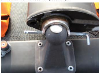
E. Attach striker bar (9) (front cross bar) between the hulls at front of boat.
