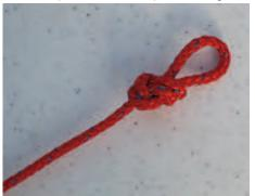
C. Then slide the loop on the lacing line over the end of the 10mm glass fibre rod. You can then begin to lace the trampoline onto the rear beam.
