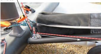
Remove the rope that is securing the double block to the spinnaker pole (this is for shipping purposes only).
