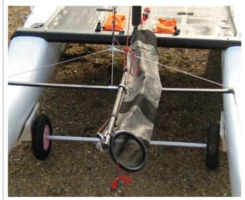
Attach velcro straps around spinnaker pole.
