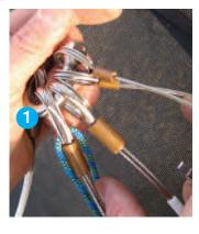
B. Attach bow shackle including rigging to crane fitting (2) located on the front of the mast section. It is important to tighten this shackle.
