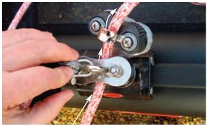
C. Then feed through eyelet on back/centre of rear beam. Tie off with a figure of eight knot.
