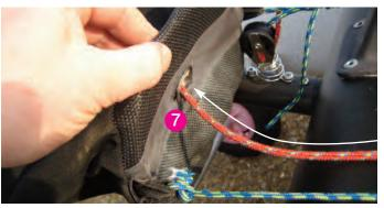
H. (8) Feed end of spinnaker halyard through the spinnaker chute until the tail comes out the front of the chute. (Tip; it is easier to do this by fishing the sinaker halyard ot of the chute with a tiler arm or similar long object in order to feed it from the back of the chute to the front).
