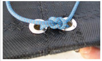
C. Tidy tail ends by tucking back down through eyelets.
