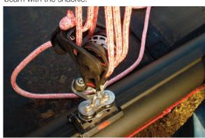
B. Feed tail end through cleat on carriage and then through double pulley block.
