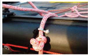
D. Then attach mainsheet system to mainsail with S hook (S).
