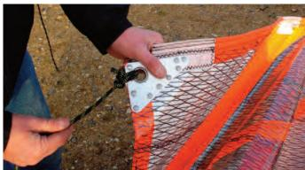
B. Hoist mainsail, feed sail into groove in mast and then raise mainsail by pulling main halyard.
