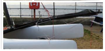
E. (1) Take line from the chute mouth and (2) tie off on to the eye on the front of the hull.
