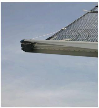
When sailing upwind you will nearly always have the outhaul pulled quite tight but you may wish to loosen it for the downwind legs. You can pre-set the "off" position by tying a large knot (or use a ball) about an inch from the cleat when the foot is pulled tight. This means you simply have to uncleat at the windward mark and it will be in about the right place for downwind sailing. Remember to pull it back on before rounding the leeward mark!
