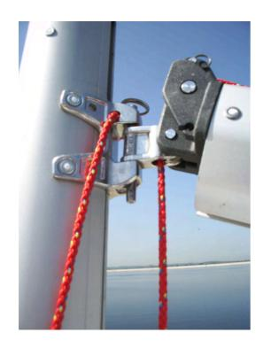
Next attach the strut to the upper fitting on the mast. Ensure the toggle is correctly orientated. See Selden info sheet.
