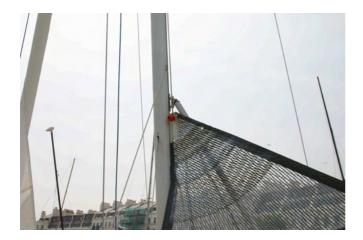
(TIP: Check the wear on the Halyard regularly, particularly where it goes over the masthead sheave. You can prevent excessive wear by moving the knot at the head every so often by adding additional overhand knots further and further down the Halyard. When you have done this a few times you will have to trim the excess knotted line to save windage).
