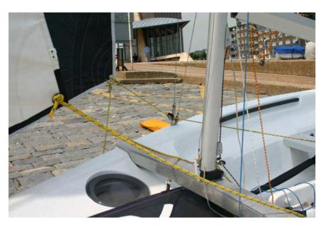
15 Undo forestay and attach to beam eye on the base of the mast.
