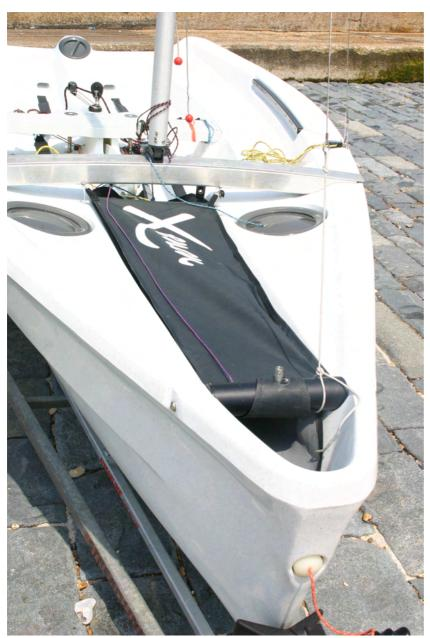
5 Attach lowers in to the adjuster plates and tie off on each side of hull.
