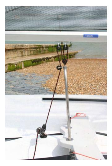
Then attach the foot of the jib to the Furler at the front of the boat (ensure the Furler is fully wound up). Attach jib head to the swivel on jib Halyard.
