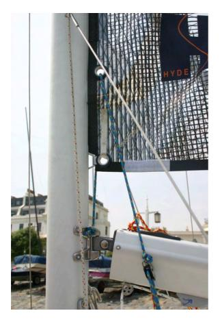
38-39 Having raised the sail, insert the slug at the back of the sail into the track on the boom.
