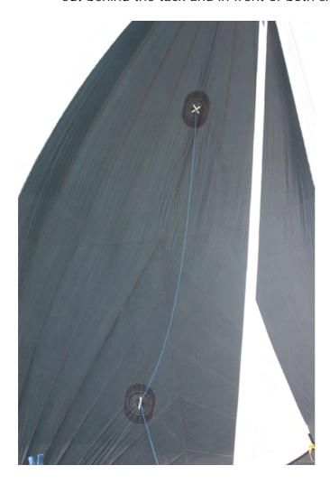
You should now be able to pull the Gennaker down into the chute, ensuring that it does not snag around the pole-end or under the bow.
