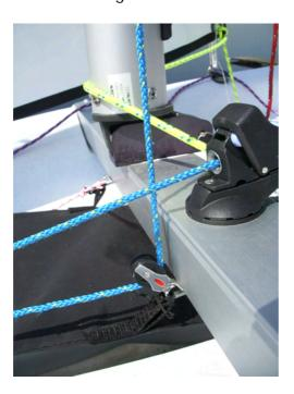
19 Then forward, around the free block located to the side of the Gennaker chute (attached to the line that pulls the pole out).
