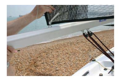
Take the control line from the sheave in the boom-end fitting and feed through the eye in the sail and back through the pulley in the boom-end. Then via the notch in the fitting underside. Tie a small knot in end.
