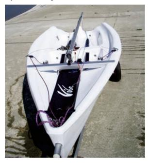
Untape all the ropes attached to the foot of mast.
