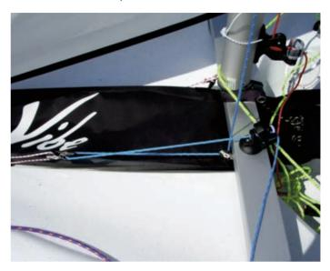
Then through the eyelet at the back of the sock. Feed it up the sock to the mouth of the chute.
