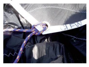
Now you have all three corners of the gennaker tied on and you can attach the downhaul. This can be tricky - and embarrassing if you get it wrong - especially if you do not notice until the first hoist or even the first gybe!
