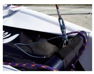
Ensure all halyards from mast are clear and not twisted or snagged.
