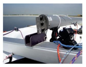
Ensure all halyards are in place at foot of mast. You may now pull the mast up using the forestay. You may require someone to lift the top of the mast.
