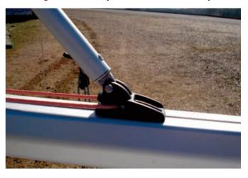
Having fixed the boom and gnav to the mast, thread the gnav control line from the fitting at the front of the boom through the cleat on the mast.
