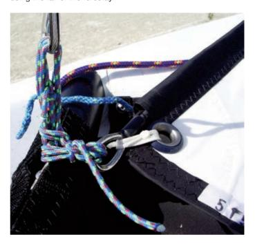
Attach jib head to the shackle on jib halyard. Pin downward.
