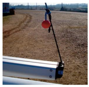
TIP: You can tie a stopper knot in halyard by the mast to support the boom while you rig.
