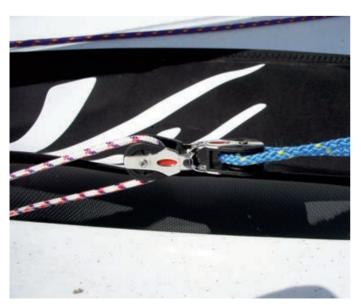
Lead the end down through the block at the front of the centerboard case. Round the back first (i.e., feed forward from the back of block).
