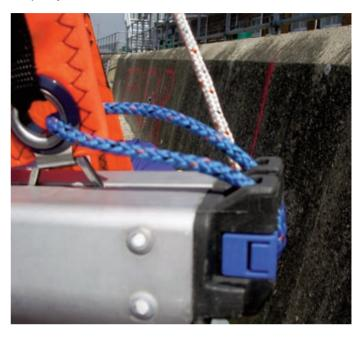
Then via the notch in the fitting underside, tie a small knot in end.
