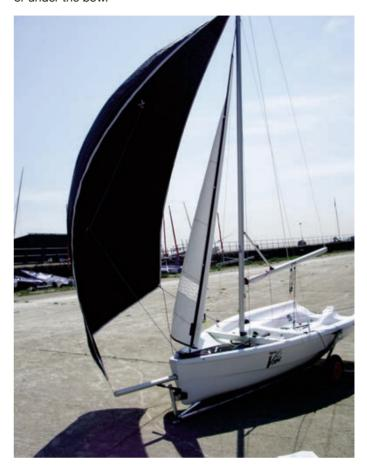
TIP: When launching the gennaker. Pull gennaker halyard from block NOT direct from chute. This will prevent wear and tear at chute opening.
