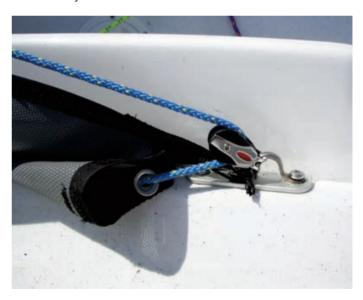
The tack line emerges from the forward end of the bowsprit. Tie a figure-of-eight knot about 6in /15cm from the end of this line and an overhand knot right at the end.
