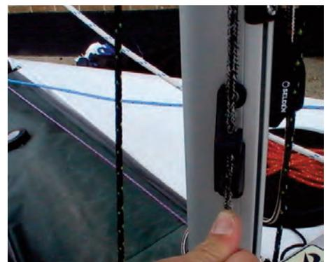
TIP: Check the halyard for excessive wear regularly, particularly where the line goes over the masthead sheave. Wear can be prevented by moving the knot at the head every so often by adding additional overhand knots.
