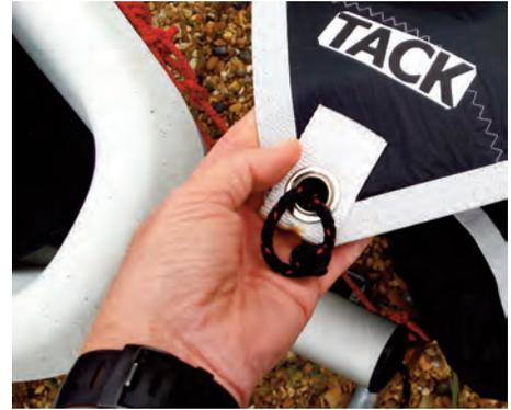
4:12 Temporarily remove the red ball from the spinnaker halyard. Then pass the end of the spinnaker halyard through the eyelet in the sail as shown.
