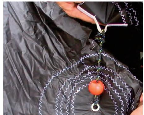
4:15 Pull on the end of the spinnaker halyard coming from the end of the spinnaker chute within the boat in order to pack the spinnaker into the chute.
