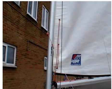
6:5 Release the main halyard from the cleat, and uncleat the gnav, and then pull on the reefing line. The foot of the sail should fold up so that the sail area is reduced.
