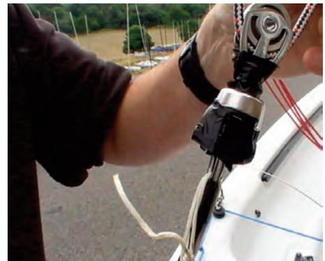
3:3 Pull the jib halyard in order to raise the jib, and then cleat the halyard off on the right side of the mast. In order to apply the most rig tension, sweat the jib halyard as shown.
