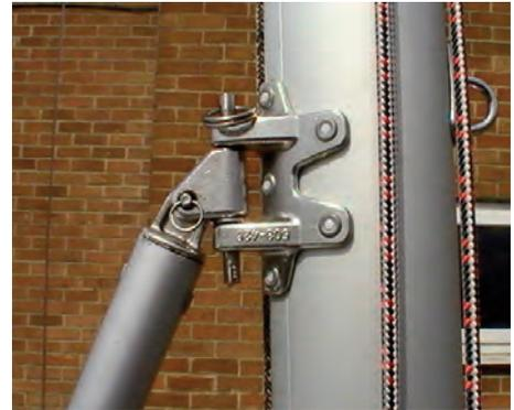
2:3 Having fixed the boom and gnav to the mast you can thread the gnav control line. This comes out from the boom at the front, and then feeds through the swivel cleat on the mast.
