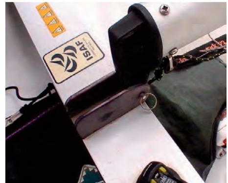
1:6 Pull the mast up using the forestay. To make it easier, someone else can lift the top of the mast.
