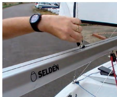
5:6 Pass the outhaul through the eyelet in the clew, and then back to the end of the boom, where the end of the outhaul should be cleated. The outhaul can be tightened at the mast end of the boom.
