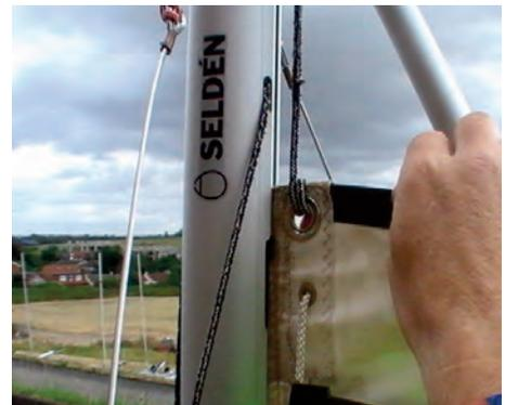
5:4 Cleat the main halyard in the cleat on the left of the mast. Sweat the halyard in order to make sure that the sail is at the top of the mast.
