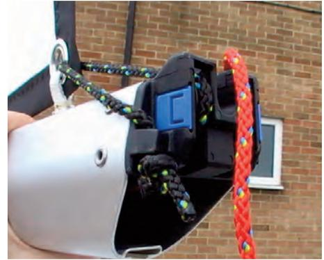
6:2 Feed the reefing line through the eyelets in the leech of the sail.
