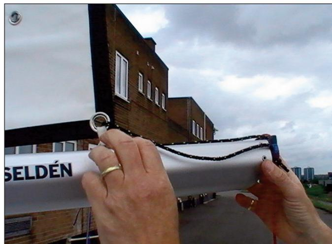
5:6 Hook the downhaul onto the sail, ensuring that it is not twisted before applying any tension.
