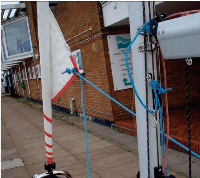
3:8 Cleat the jib furler off in the cleat underneath the crossbeam.
