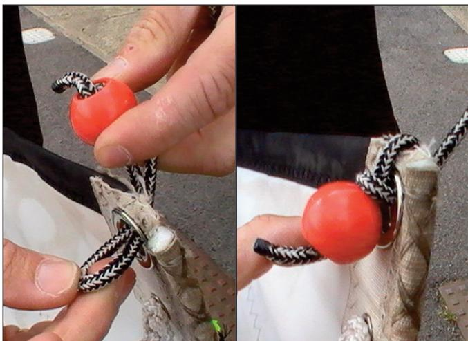
5:3 Raise the sail by placing the bolt rope in the cut out of the mast just above the boom, and then pulling on the halyard. NB: It may be easier to raise with two people, as one can pull the halyard while the other can feed the luff of the sail into the mast. Ensure that the boat is still head to wind before the sail is raised
