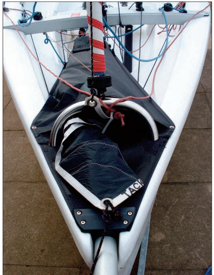
5:1 Tie the flotation panel to the top of the mainsail by passing the white lines through the eyelets in the sail and secure with a figure of eight knot.
