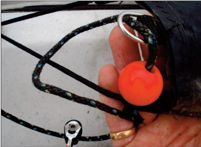
4:8 Pass the line up the chute, feeling for the ball inside, until it reaches the opening at the front.
