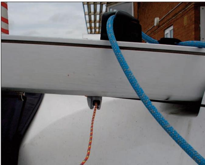
3:9 Now tie the lowers onto the shackle on the fitting attached to the shroud fitting.
