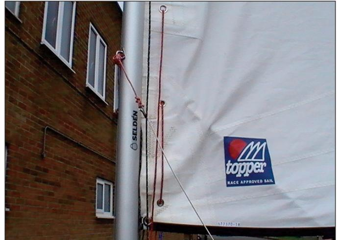
6:5 Release the main halyard from the cleat, and uncleat the gnav, and then pull on the reefing line. The foot of the sail should fold up so that the sail area is reduced. Once the desired sail area is achieved, cleat the reefing line and main halyard, and re-apply gnav tension.
