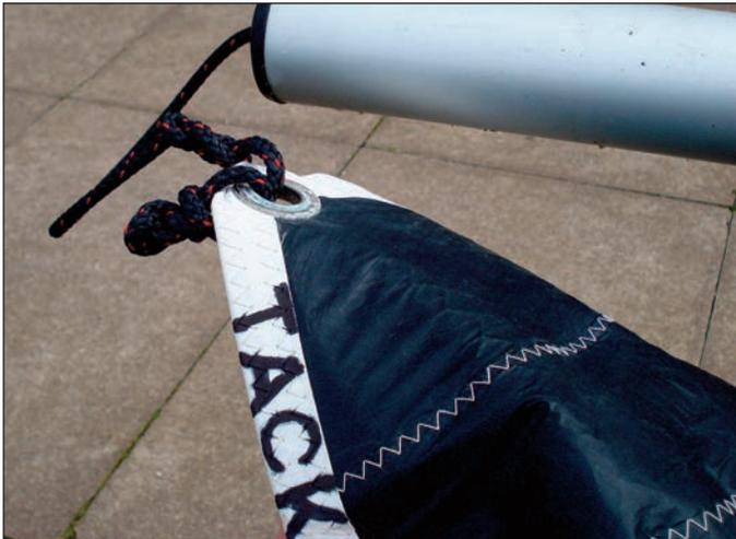
4:12 Temporarily remove the red ball from the gennaker halyard. Then pass the end of the gennaker halyard through the rings on the sail as shown
