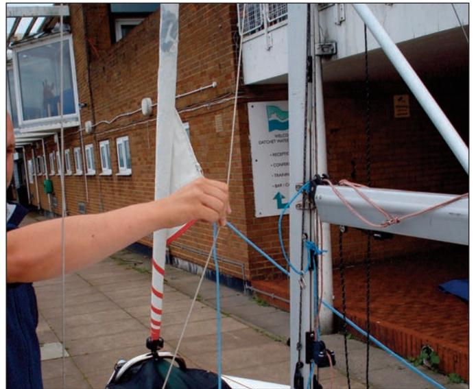
The tail of the jib halyard can be stowed in the pocket on top of the gennaker chute. It is not advisable to leave the jib up overnight, and always take the jib tension off when the boat is not being sailed.
