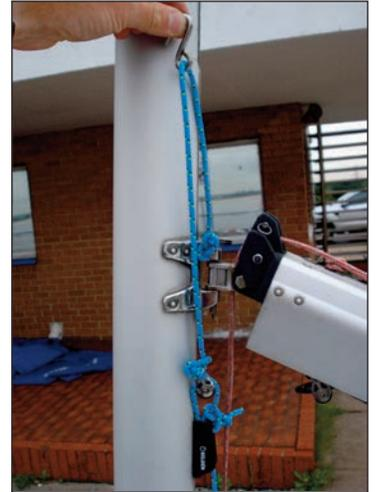
2:4 Now thread the mainsheet. Starting from the centre cleat on the hull (NB: ensure the ratchet clicks when the rope is pulled in), go up to the rear block, and thread the line from back to front. Then go to the pulley on the top of the centre block, and thread it from back to front. Then go to the front pulley on the boom, and thread it from front to back.
