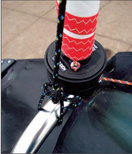
4:2 Take the other free end of the halyard and feed it through the pulley on the front of the crossbeam.
