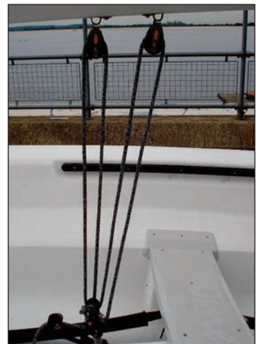
2:5 The mainsheet goes to the pulley on the deck and through the hole in the centre of the pulley. Tie a stopper knot to prevent the line unthreading. Tie a figure of eight knot in the loose end so that the boom does not hit the shroud when sheeting out.
