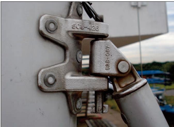
2:3 Having fixed the boom and gnav to the mast you can thread the gnav control line. This comes out from the boom at the front, and then feeds through the swivel cleat on the mast. TIP: You can tie a stopper knot in the end of the main halyard and then attach this to the end of the boom, so that the boom is held up while the rest of the rigging is completed.
