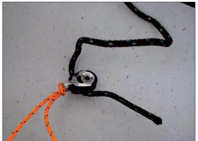
4:6 Pass the halyard through the eyelet in the bottom of the gennaker chute.
