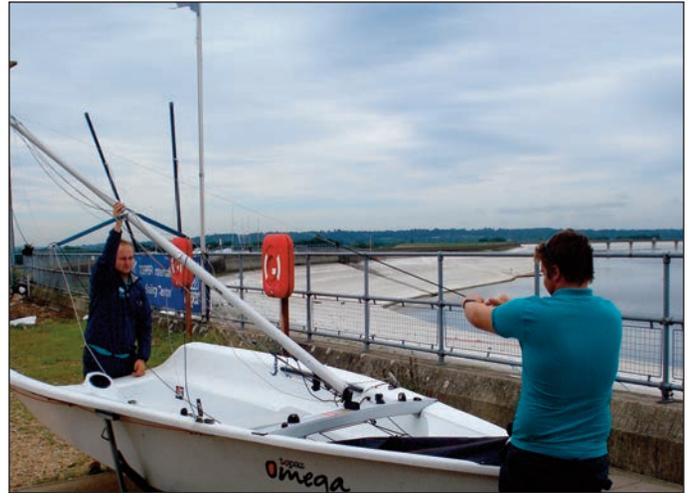
1:7 Having pulled the mast upright, secure the forestay around the stainless steel chute mouth bar. Ensure all halyards are clear and not twisted.
