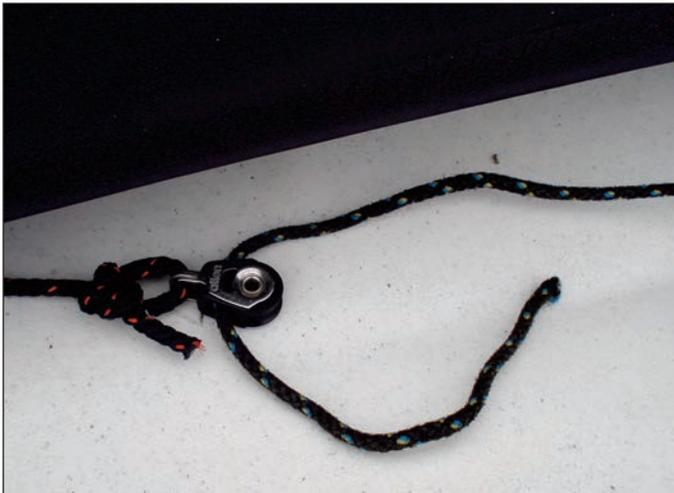
4:4 Take the halyard through the Spinlock Cleat that is mounted on top of the crossbeam.
