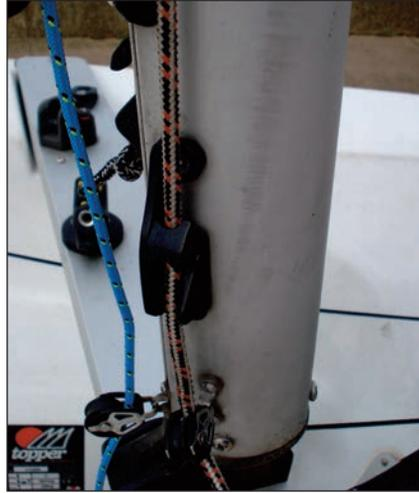
3:4 Once the rig tension has been applied, the forestay can be moved back from the bar at the front and then tied off to the mast.
