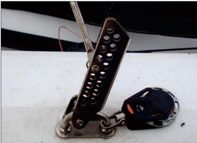
1:5 Fix the base of the mast to the mast step on the cross beam with the pin and ring from the mast step.
