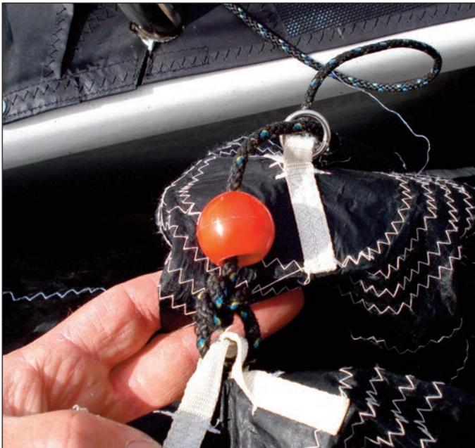
4:15 Pull on the end of the gennaker halyard coming from the end of the gennaker chute within the boat in order to pack the gennaker into the chute.
