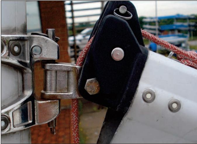
2:2 Next attach the strut to the upper fitting on the mast. Ensure the toggle is correctly orientated as per the Selden/Superspar info sheet. Fix the gnav strut carriage on top of the boom, although this should already be fixed for you.
