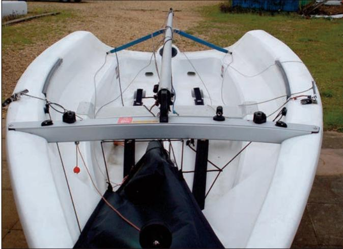
1:4 Attach the shroud adjusters to the shroud eyes each side, on approximately the 5th hole down on the stern side.
