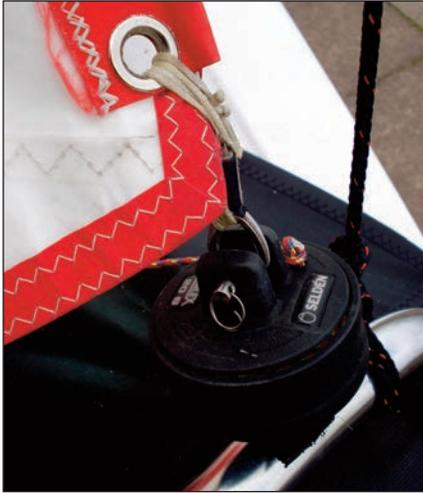
TIP: Wrap some electrical tape around the furler. This will protect the gennaker from the sharp split ring and help to prevent rips in the sail.
