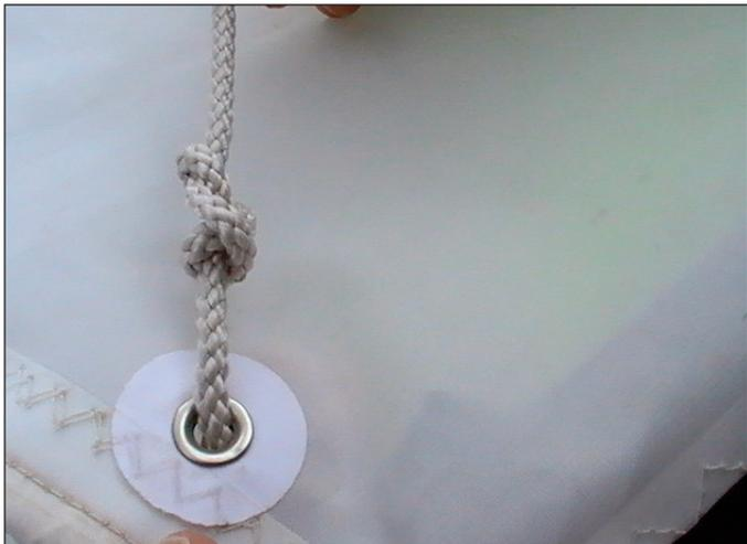
5:2 Tie the free end of the main halyard to the eyelet on the top of the mainsail.
