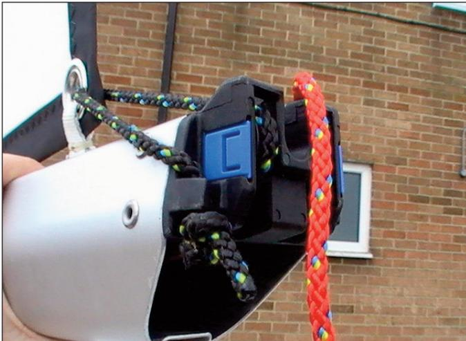
6:2 Feed the reefing line through the eyelets in the leech of the sail.
