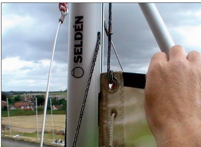
5:4 Cleat the main halyard in the cleat on the left of the mast. Sweat the halyard in order to make sure that the sail is at the top of the mast. This is done by holding the halyard just above the cleat and then pulling away from the mast at 90 degrees. Then re-cleat the halyard until the sail is at the top of the mast.
