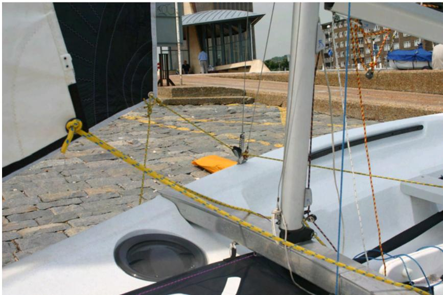
15 Undo forestay and attach to beam eye on the base of the mast.
