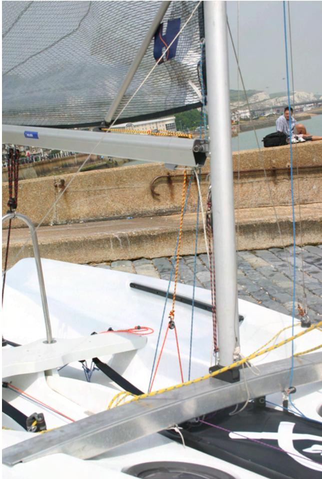
Attach main Halyard to the end of the boom.
