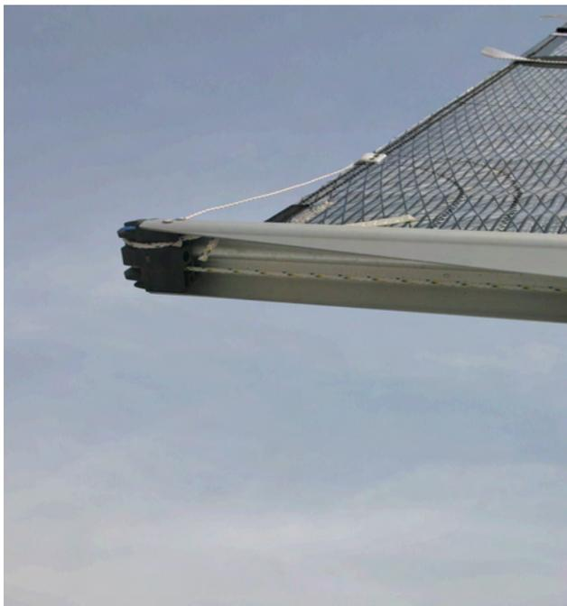
When sailing upwind you will nearly always have the outhaul pulled quite tight but you may wish to loosen it for the downwind legs. You can pre-set the "off" position by tying a large knot (or use a ball) about an inch from the cleat when the foot is pulled tight. This means you simply have to uncleat at the windward mark and it will be in about the right place for downwind sailing. Remember to pull it back on before rounding the leeward mark!
