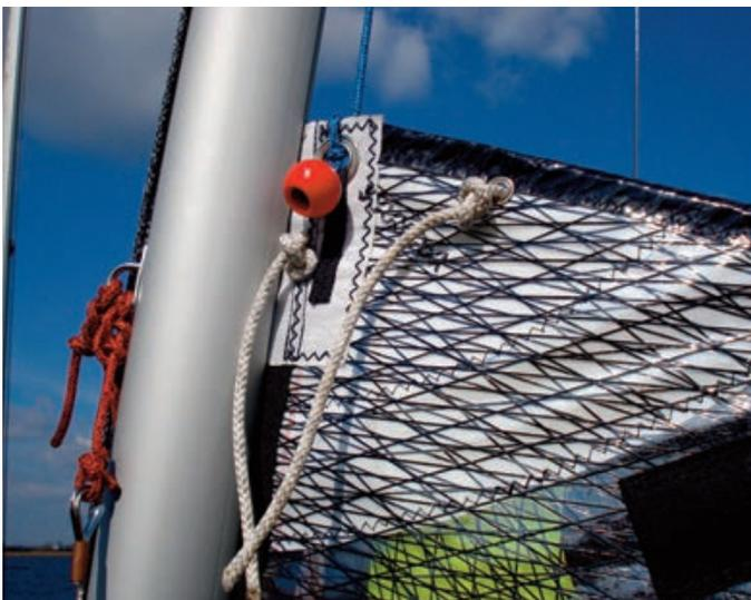
Before raising the sail, insert the slug at the back of the sail into the track on the boom.
