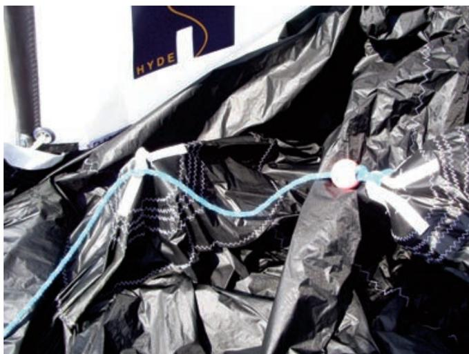
You should now be able to pull the gennaker down into the chute, ensuring that it does not snag around the pole-end or under the bow.
