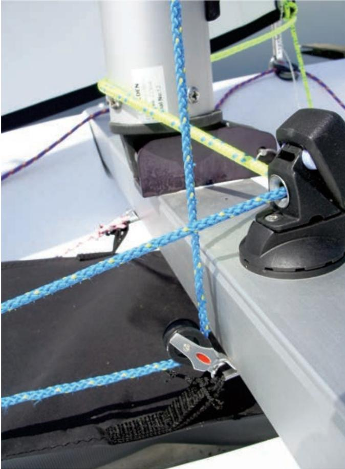
Then forward, around the free block located to the side of the gennaker chute (attached to the line that pulls the pole out).
