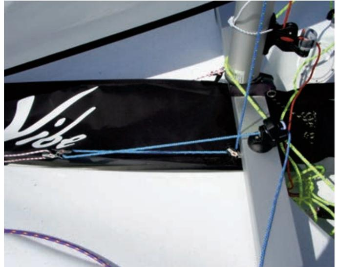
Then through the eyelet at the back of the sock. Feed it up the sock to the mouth of the chute.
