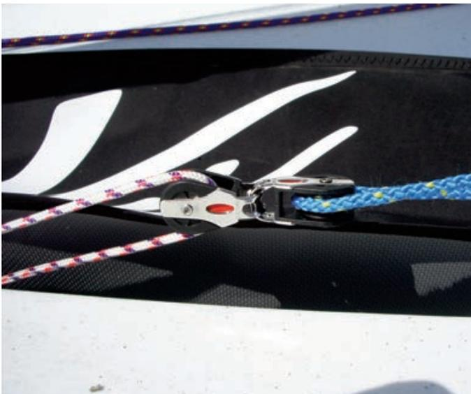
Lead the end down through the block at the front of the centerboard case. Round the back first (i.e., feed forward from the back of block).
