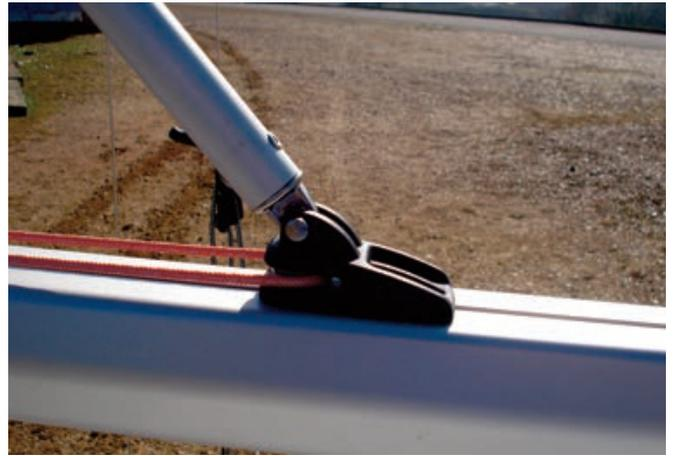
Having fixed the boom and gnav to the mast, thread the gnav control line from the fitting at the front of the boom through the cleat on the mast.
