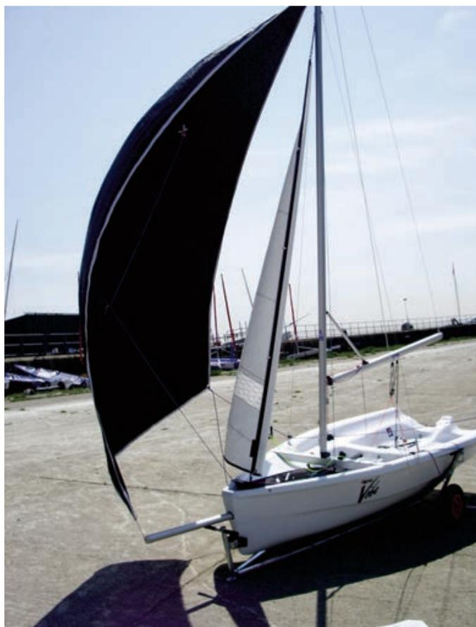
**TIP: When launching the gennaker. Pull gennaker halyard from block NOT direct from chute. This will prevent wear and tear at chute opening.**
