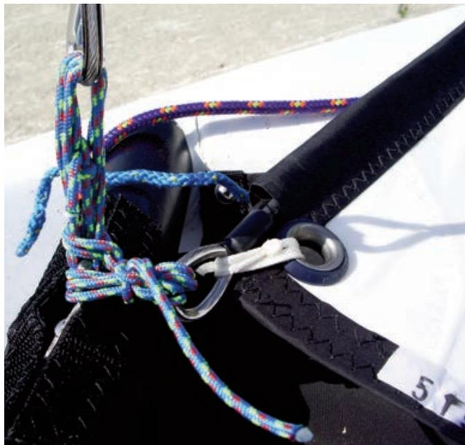
Attach jib head to the shackle on jib halyard.
