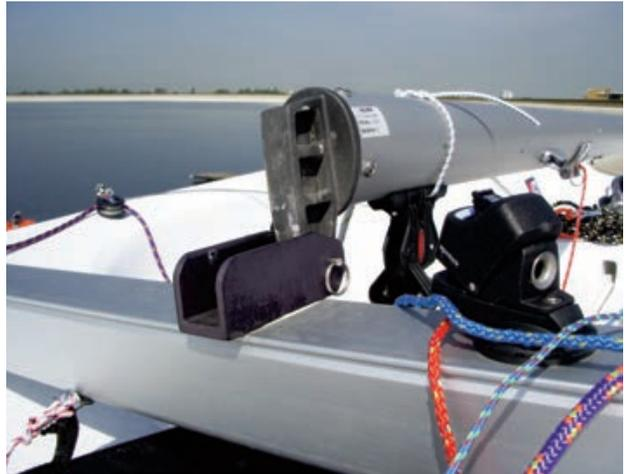
Ensure all halyards are in place at foot of mast. You may now pull the mast up using the forestay. You may require someone to lift the top of the mast.
