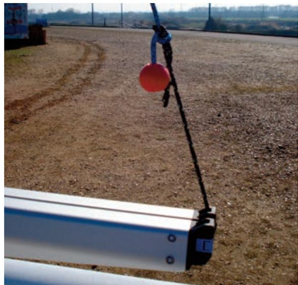
**TIP:** You can tie a stopper knot in halyard by the mast to support the boom while you rig.
