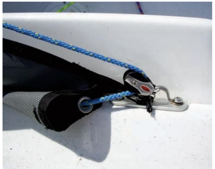
The tack line emerges from the forward end of the bowsprit. Tie a figure-of-eight knot about 6in /15cm from the end of this line and an overhand knot right at the end.
