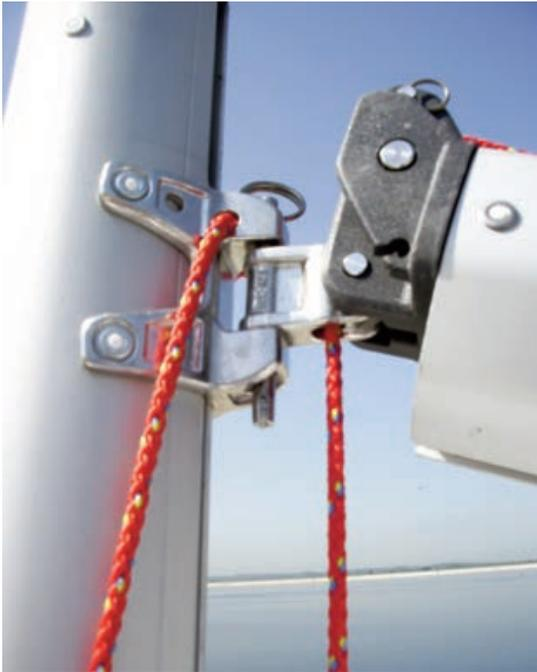
Next attach the strut to the upper fitting on the mast. Ensure the toggle is correctly orientated.
