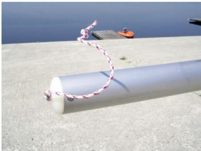
Pull the pole right out: the easiest way to do this is to tie off the top end of the gennaker halyard and pull on the other end. This should launch the pole by pulling the single block back down the boat. Ensure that the pole is right out. The lines should be pre-set to the correct position - i.e. the pole goes right out; when it is out the figure-of-eight knot in the tack line is pulled right to the end of the pole.
