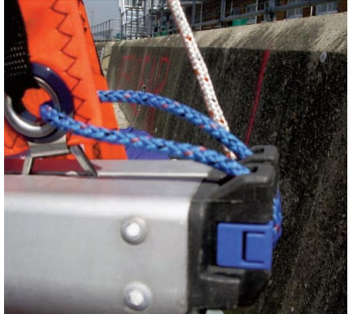
Then via the notch in the fitting underside, tie a small knot in end.
