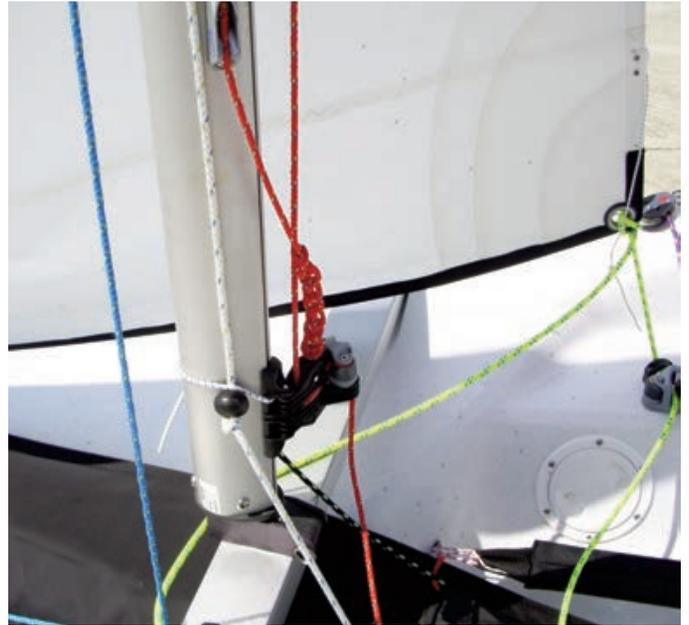
**TIP:** Check the wear on the halyard regularly, particularly where it goes over the masthead sheave. You can prevent excessive wear by moving the knot at the head every so often by adding additional overhand knots further and further down the halyard. When you have done this a few times you will have to trim the excess knotted line to save windage.
