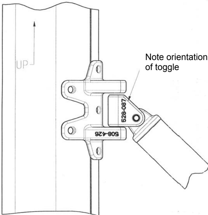
Fix the gnav strut to the carriage on the top of the boom. The carriage should already be fixed to the boom for you.
