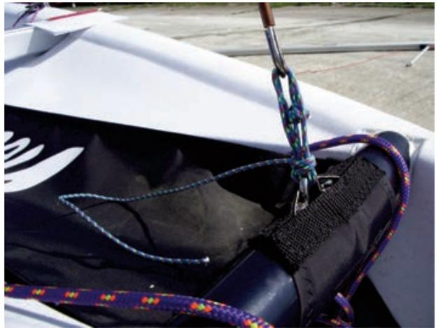
Ensure all halyards from mast are clear and not twisted or snagged.
